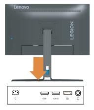
3. Connect one end of the DP cable to the DP connector on the back of the computer, and the other end to the DP connector on the monitor. Lenovo recommends that customers who require to use the Display Port input on their monitor purchase the "Lenovo Display Port to Display Port cable 0A36537". www.lenovo.com/support/monitoraccessories
