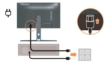
7. Connect the cables with cable clip.
