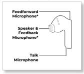
\*Feedforward and feedback microphones are used for noise control modes. For more, see **Set the noise control modes**.
