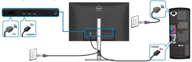
Connecting/ disconnecting the monitor for RJ45 cable (optional) and Power cable
