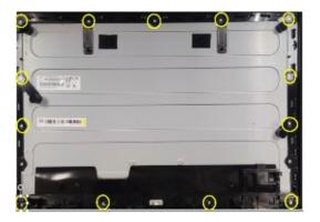
S16 (Screw Torque: 4.5-5.0 kgf) Tear off two acetate tapes from the convex holes on "Panel
