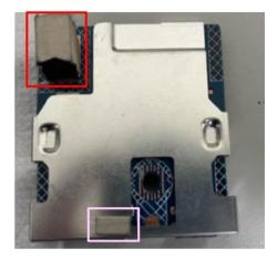
S11 Disassemble "USB board" from "USB Shielding"
