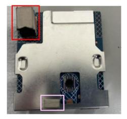
S14 Assemble "USB board" with "Middle Frame"
