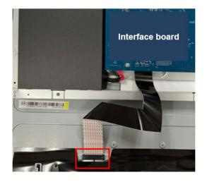
S15 Unlock 13 screws to disassemble "Middle Frame" from "Panel"
