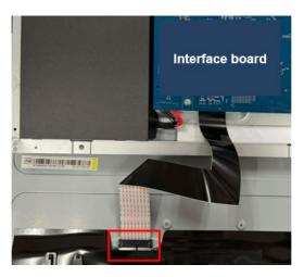
S9 Attach a yellow tape to fix "LVDS FFC" on "Panel"
