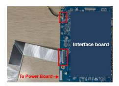
**S3** Insert "Power board wire" to "Interface board" and assemble "Interface board" to "Main Shielding"
