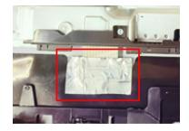
S11 Attach 2 conductive tapes on "Main Shielding and "Panel"
