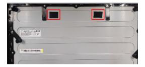
S17 Disassemble "MYLAR" from "Main Shielding"
