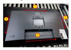
Lift the rear cover up carefully. Disconnect the joystick cable from the connector of the interface board, and then remove the rear cover.
