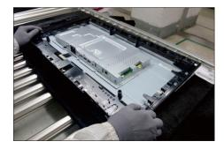
Use a Philips-head screwdriver to remove 2pcs screws for unlocking the bracket chassis with the panel.
