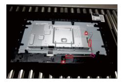
S12 Lift up the middle frame away from the panel module and put it aside.
