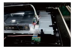
Put the rear cover into a fixture jip, then release the key cable by tearing off the tapes. Use a Philipshead screwdriver to remove 1pcs screws for unlocking the joystick key board with the rear cover.
