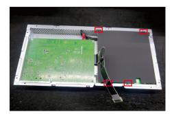
Use a Philips-head screwdriver to remove 5pcs screws for unlocking the power board and interface board, and then release all the cables from the hooks.
