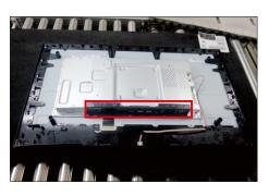
S11 Disconnect the panel lamp cable from the connectors of the panel and interface board, then tear off the tapes and release the lamp cable from the hook of middle frame.
