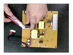
S18-4 Take out bulk cap. pin solder with soldering iron and absorber.
