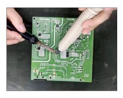
S18-5 Lift the bulk cap. up and away from the PCB.
