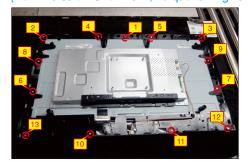
S10 Release the IO cover from the hooks of the main bracket chassis and put it aside.
