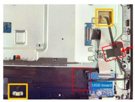
Tear off a black tape from "USB board FFC" and "Panel
