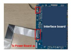
Insert "Power board wire" to "Interface board" and assemble "Interface board" to "Main Shielding"
