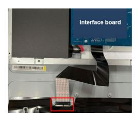
S14 Unlock 13 screws to disassemble "Middle Frame" from "Panel"
