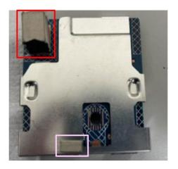
S11 Disassemble "USB board" from "USB Shielding"
