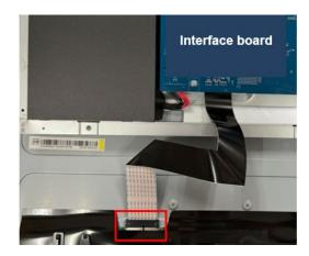
Attach a yellow tape to fix "LVDS FFC" on "Panel"
