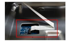
Unlock 3 screws to disassemble "Control board" from "Rear Cover"
