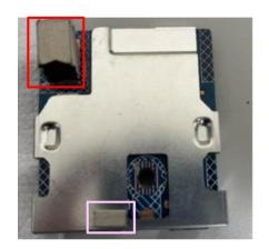
S11 Assemble "USB board" with "Middle Frame"
