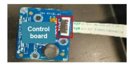
S13 Assemble "Control board" to "Rear Cover"
