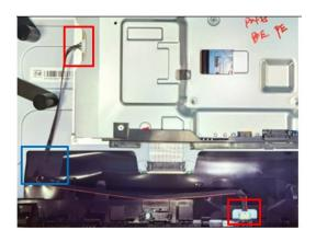
Assemble "USB board" with "USB Shielding"
