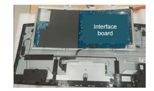
S19 Unlock 19 screws to disassemble "Middle Frame" from "Panel"
