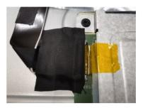
S9 Place "Main Shielding" on "Panel" and lock 4 screws to fix it on "Panel"
