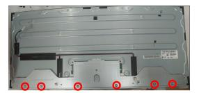
S21 Disassemble "MYLAR Power" from "Main Shielding"
