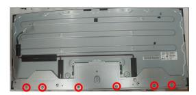
S21 Disassemble "MYLAR Power" from "Main Shielding"
