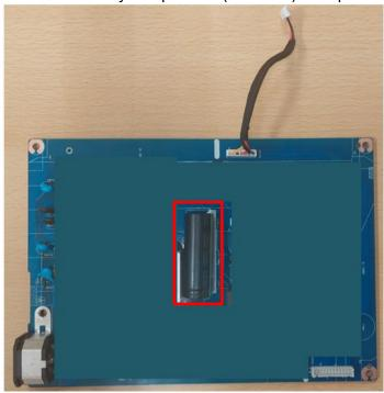
S25-1 Cut the glue between bulk cap. and PCB with a knife
