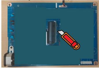
S25-2 Ensure cutting path within the glue, don't touch bulk cap. or PCB
