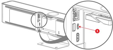
Image 4-10 Where to connect the USB-C cable
