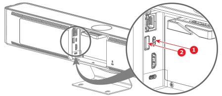
Image 4-17 Where to connect the USB-C cable or dongle and the USB-A cable (only for touch screens)
