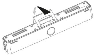
Image 4-2 Tilt direction for the wall stand
