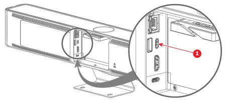
Image 4-11 Where to connect the USB-C cable
