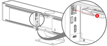
Image 4-20 Where to connect the LAN cable
