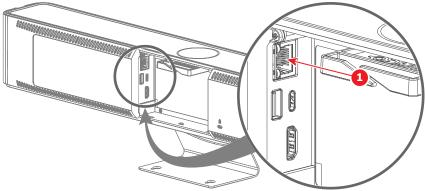
Image 4-19 Where to connect the LAN cable
