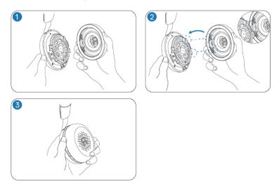
**NOTE:** Ensure that the R and L markings on the ear cushion are correctly positioned when replacing.
