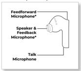
\*Feedforward and feedback microphones are used for noise control modes. For more, see **Set the noise control modes**.
