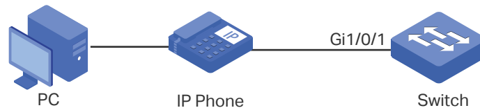
Figure 6-1 LLDP-MED Network Topology
