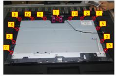
Lift up the middle bezel away from the pane module, **S18** then put it on a cushion foam for later disassembling.
