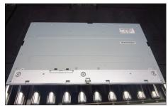
Remove the Mylar tape from the hooks of the bracket chassis.
