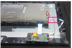
Use a Philips-head screwdriver to remove 2pcs screws for unlocking the middle frame with panel module and front bezel.
