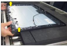
Use a Philips-head screwdriver to remove 4pcs screws for unlocking the left and right Mic boards with the middle frame, then release the two Mic S19 boards away from the middle frame.
