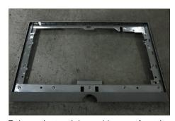
Release the touch key cable away from the panel, then disassemble the front bezel with the panel, then S20 tear off the mylar tape and release the touch board.
