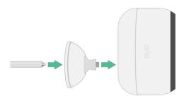
Note: The Essential Outdoor Camera has one mounting hole located at the back of the camera near the charging port.
