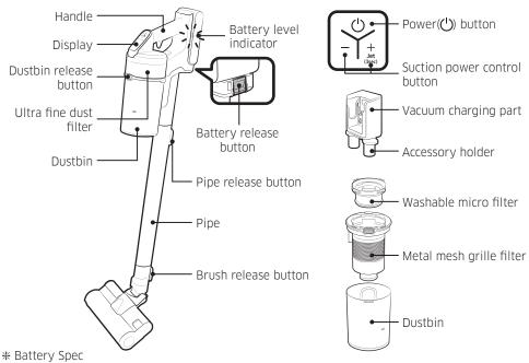
VS20B75\*\*\*\* Series : Lithium-ion 21.6 V, 1800 mAh, 6 cell
