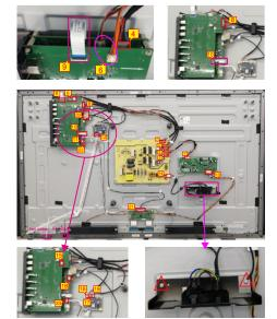
Use a screwdriver to remove 4pcs screws for unlocking the two speakers. (Torque: 4.5kgf±0.5)
