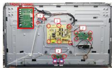
Use a screwdriver to remove 30pcs screws
