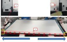
S22 Remove 1pcs DEBF film, 1pcs Diffuser film, 1pcs LGP, 1pcs Reflector film away from the back bracket.
