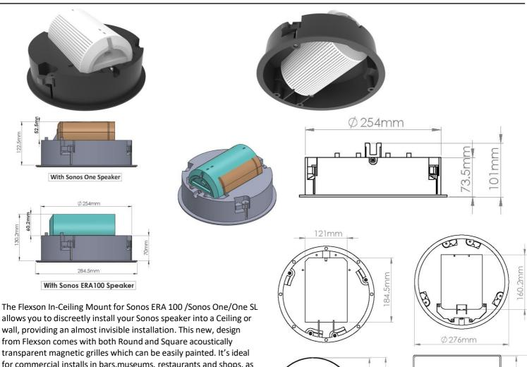
allows you to discreetly install your Sonos speaker into a Ceiling or wall, providing an almost invisible installation. This new, design from Flexson comes with both Round and Square acoustically transparent magnetic grilles which can be easily painted. It's ideal for commercial installs in bars, museums, restaurants and shops, as well as for home use.
