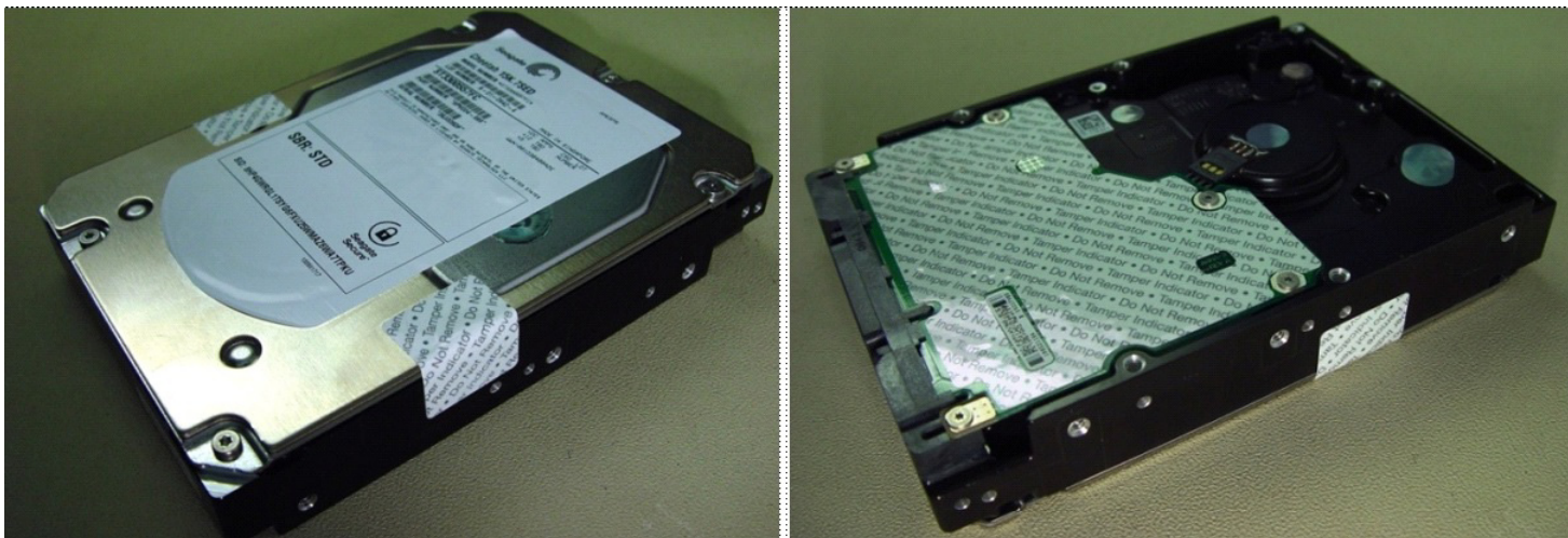
Figure 5. Example of FIPS tamper evidence labels.
