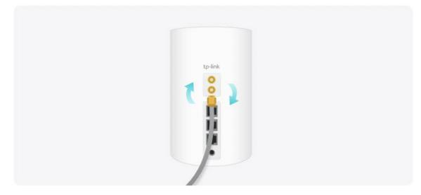
3. Open the Deco app, go to More > External Antennas and enable External Antennas. When enabled, the external antennas will replace part of the internal antennas.
