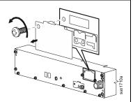
Onnect the battery connector cables and communication cables.
