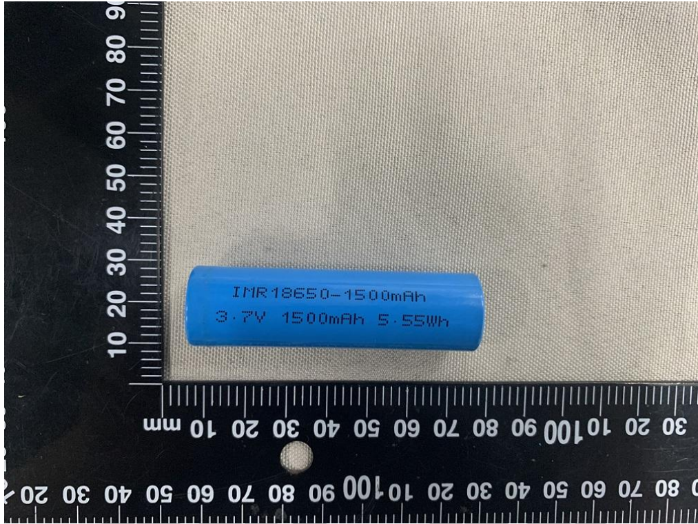
Cell (IMR18650-1500mAh, 3.7V, 1500mAh, 5.55Wh)
