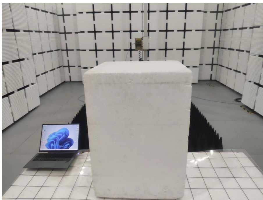
Set-up for Transmitter & Receiver Spurious Emissions, Above 1GHz
