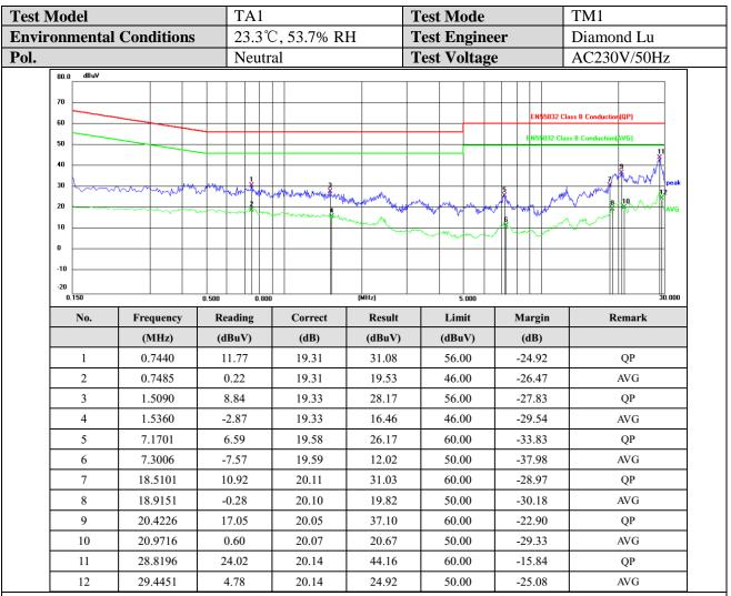
Note: For conducted emission and radiated emission test, a power supply of 230VAC and 120VAC was used for testing respectively, and only recorded the worst case of 230VAC.
