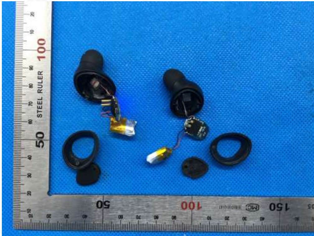
Fig.11 – open view of headset
